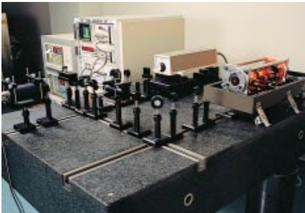
Iodine Absorption Stabilized He-Ne Laser as the standard for length measurement (At Tsukuba Calibration Center)
