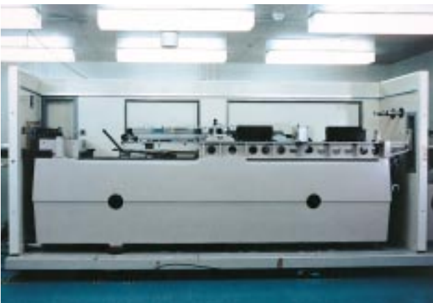
Interferometer as the standard for Linear Scale calibration (At Kiyohara Plant)
