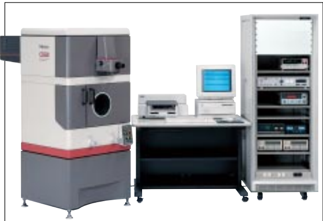
Interferometer as the standard for Gauge Block calibration (At Miyazaki Plant)
