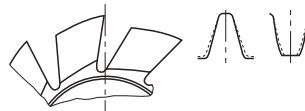
Fig. 11: Positional deviation of the cutting face a) Faulty, positive cutting face position b) Elongated cutter tooth c) The workpiece tooth becomes thicker at the head, tip contact The broken-line contours indicate the theoretically correct profile of the cutter- or workpiece tooth.
